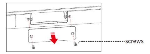
Insert the SDM-S into the port on the rear of the panel until firmly seated, using the 2 screws to secure it.
