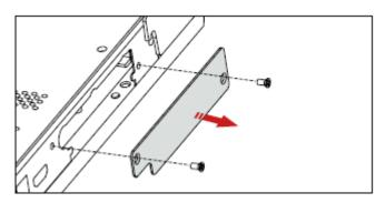
Insert the Wi-Fi Module into the port on the rear of the panel until firmly seated, using the 2 screws to secure it.
